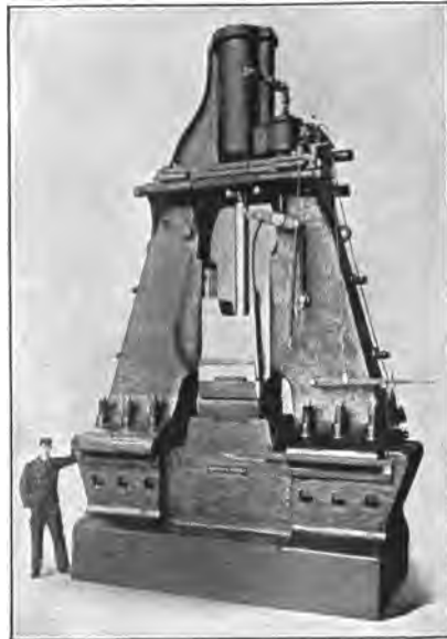
Fig. 154. Typical Steam Hammer Courtesy of Niles-Bement-Pond Company.
